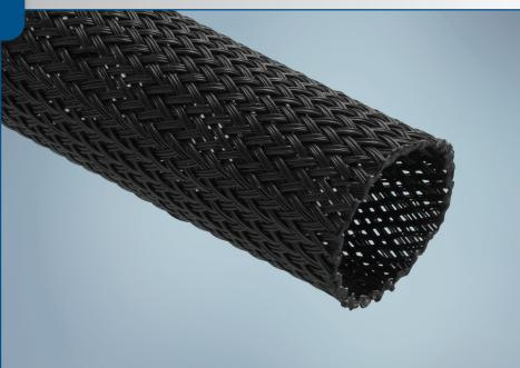
**FlexGuard® 2130** is a lightweight and flexible braided sleeve designed to provide mechanical protection for most common automotive applications. Constructed of PA (polyamide) monofilament guard strands and PET (polyethylene terephthalate) support strands, this dual-monofilament blend provides an excellent balance of abrasion protection, temperature resistance, and installability.
