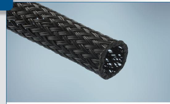
**FlexGuard® 2129** is a lightweight, expandable sleeve designed to provide mechanical protection for electrical distribution systems, hoses and cable assemblies. A dual monofilament construction that blends larger nylon monofilament guard strands with polyester support strands, provides an excellent balance of key features including abrasion resistance, flexibility, expandability and self-recovery.
