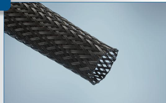
**FlexFit® 2112** is an expandable sleeving specifically designed for the abrasion protection of automotive wire harnesses, cables, tubings and hoses. Its specific structure combines both a high coverage ratio and a high expansion ratio which enables installation over long lengths even after the fitting of end connectors. It also allows a large number of diameters to be covered with a limited range of sizes.
