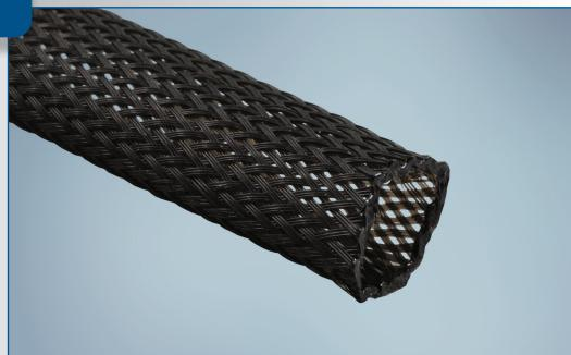
**FlexFit® 2010** is a tough, lightweight oversleeve designed to protect cables assemblies, hoses and wire harnesses from chafing, cutting and abrading. The open weave construction enables each size to expand to fit several application shapes and sizes. The construction also makes it highly flexible and resistant to trapping water, heat and humidity.
