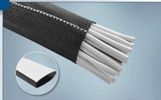
FastWrap™ 2305 is an open sleeve designed to offer a high level of component protection. Constructed with a combination of monofilament and multifilament yarns, FastWrap 2305 also incorporates an adhesive tape system to ensure secure closure of the sleeve.
