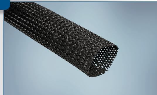
**Expando® PT & Expando® PT Plus** are tough, lightweight oversleeves used to protect cable assemblies, hoses and wire harnesses from chafing, cutting and abrading. The open-braid construction of Expando products enables each size to expand to fit several application shapes and diameters. This open-textile construction also makes them highly flexible and resistant to trapping water, heat and humidity.
