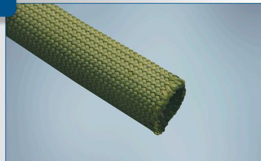
**Expando® HTNS-L/HO** is a thin wall braided sleeve manufactured from the meta-aramid Nomex®. Its highly expandable structure allows easy installation over long lengths even after the fitting of end connectors with a limited range of product sizes.
