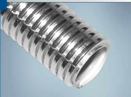
**ConvoShield**<sup>®</sup> is a reflective convolute sleeve designed to provide thermal protection for components in radiant heat environments. Composed of a high temperature nylon 4,6 polymer base substrate and a highly reflective coating, ConvoShield provides protection for wires, cables and hoses in applications that have radiant heat source temperatures as high as 538°C (1000°F).
