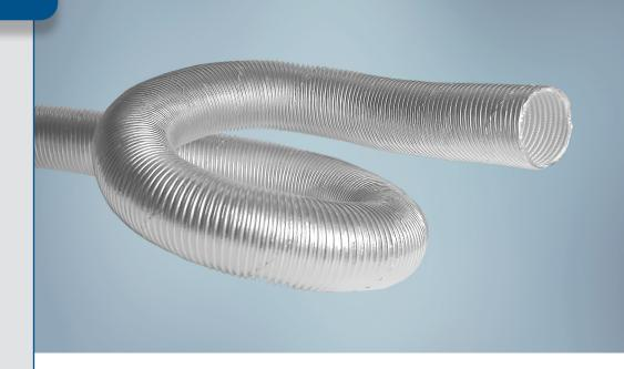
**Clevaflex® F-A** is a reflective corrugated tube designed to provide thermal protection for components in radiant heat environments. Its multi-ply construction of aluminum laminated fiberglass coupled with an aluminum foil exterior also allows for good insulation to components requiring stable temperatures for optimum performance efficiency.
