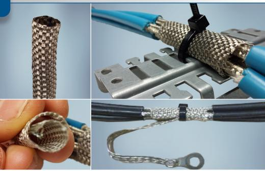
**C-Ground™ SW 125** is a wrap-around grounding solution allowing high conductivity between shielded wires. C-Ground™ SW 125 is manufactured from UL 94 V0 rated PPS monofilaments and tin plated copper wires according to EN13602.
