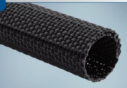
**TwistWrap® 2403** is a self-wrapping sleeve designed to enable fast and easy wire harness bundling. Woven of both monofilament and multifilament polyester yarns the product is both flexible and lightweight. The polyester construction eliminates problems associated with trapped heat and humidity. The combination of materials also enables the product to provide a level of abrasion protection for the wire bundle.
