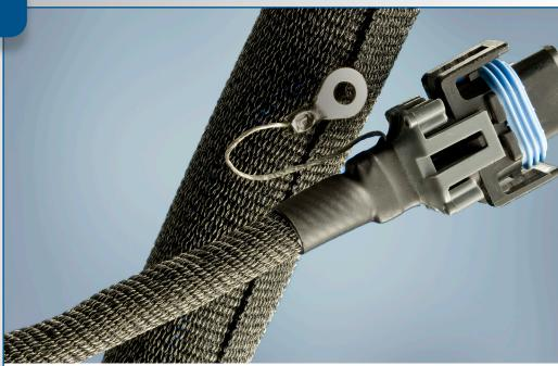
**TwistTube® 2473** is a family of self-wrapping sleeves designed to provide electromagnetic (EM) screening attenuation. Tinned copper wire is combined with polyester yarn to create a wrappable product that offers flexibility and consistent shielding protection. The product features an acrylic/silicone coating to prevent end fray and enable cold cutting to specific application length.
