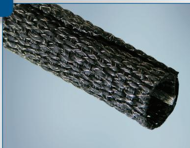
**TwistTube® 2472** is a self-wrapping sleeve designed to provide >30dB of electromagnetic (EM) screening attenuation. 316L fine stainless steel wire is combined with polyester yarn to create a wrappable product that offers flexibility and consistent shielding protection in corrosive environments. The product features an acrylic/silicone coating to prevent end fray and enable cold cutting for specific product lengths.
