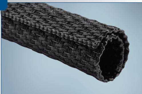
**TwistTube® 2426** is a self-wrapping sleeve designed to provide excellent edge abrasion protection and noise suppression. Woven of both monofilament and multifilament polyester yarns the product offers a high level of component protection and is both flexible and lightweight. The polyester construction eliminates problems associated with trapped heat and humidity and also eliminates operator skin irritation during assembly.
