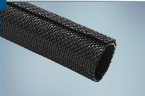
**TwistTube® 2420F** is a self-wrapping sleeve designed to provide abrasion protection and acoustical noise suppression. Woven of both monofilament and multifilament polyester yarns the product offers a high level of component protection and is both flexible and lightweight. The polyester construction eliminates problems associated with trapped heat and humidity and also eliminates operator skin irritation during assembly.
