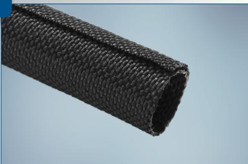
**TwistTube® 2420** is a self-wrapping sleeve designed to provide abrasion protection and acoustical noise suppression. Woven of both monofilament and multifilament polyester yarns the product offers a high level of component protection and is both flexible and lightweight. The polyester construction eliminates problems associated with trapped heat and humidity and also eliminates operator skin irritation during assembly.
