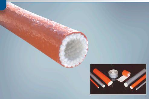
**Thermotubix**® is a thickwall braided fiberglass sleeving coated with a specially compounded, flame retardant silicone rubber. This product can be easily installed on cables and hoses and expands to pass over fittings and couplings.
