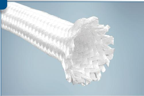
**Thermojacket® T** is constructed of braided high bulk fiberglass yarn. These yarns provide a heavier wall thickness with only a modest weight increase over other Thermojacket products. Thermojacket T provides excellent insulation properties and withstands continuous heat exposures to +538°C (+1000°F).
