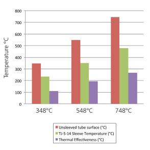
Note: Thermal effectiveness is the difference between the unsleeved and sleeved tube surface temperatures
