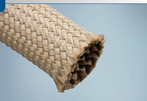
**ThermoJacket®** R sleeving is constructed of braided fiberglass. Use of an uncoated fiberglass grade results in slick, cloth-like surfaces both inside and outside of the sleeve attributing to the low friction factor of the product.
