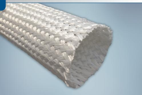
**ThermoJacket® C** is an uncoated, unsaturated sleeving braided from Nextel\* 312 ceramic fibers. ThermoJacket C retains strength and flexibility at continuous temperatures up to 1204°C (+2200°F) and offers significant protection against short term exposures at +1426°C (+2600°F).
