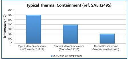
Note: Thermal Containment = Pipe Surface Temperature - Sleeve Surface Temperature.
