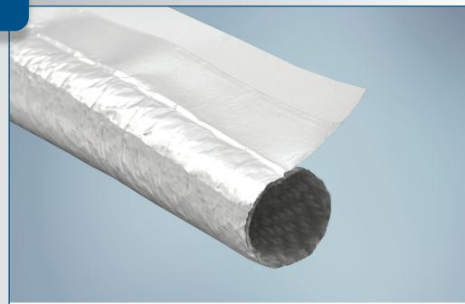
Therm-L-Wrap™ is a self-wrapping, reflective sleeve designed to provide thermal protection for both radiant and convective heat applications. Composed of a woven fiberglass base fabric and a lamination of aluminum foil, the product can withstand convective heat soaks up to +200°C (+392°F) and simultaneously protect critical components from radiant or reflected heat.
