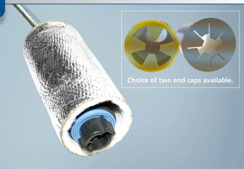
**Therm-L-Gard<sup>™</sup> V** is an aluminized, high bulk sleeve designed to provide thermal protection in high temperature environments. The outer layer is composed of an aluminum and glass fabric with the inner layer being composed of non-woven polyester.
