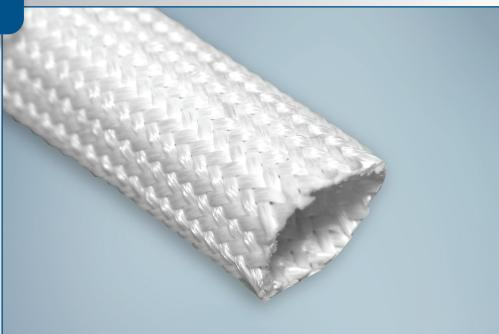
**TST/TSX** is a high temperature resistant, multifilament pure silica fibre (>99,8%) braided sleeving. It has a continuous working temperature of -60°C to +950°C.
