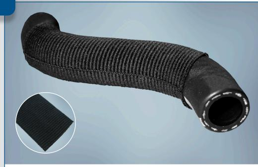
ShrinkGard™ 2800 is a highly flexible, woven sleeve constructed of polyester and polyethylene that provides good abrasion resistance for rubber hoses and tubing applications. The product offers a shrinkage up to 60% which allows ShrinkGard 2800 to accommodate a variety of diameters and sizes. The soft construction of ShrinkGard 2800 is ideal when handling the product during installation.
