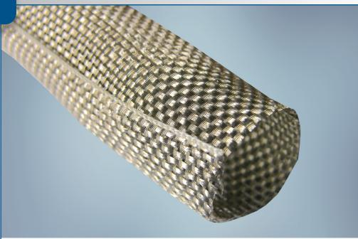
**ROUNDIT® V0 EMI** is a wrap-around sleeving designed for high performance EMI shielding of wire and cable bundles. ROUNDIT V0 EMI is manufactured from UL 94 V0 rated PPS monofilaments and nickel plated copper wires class 4 according to ASTM B-355.
