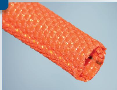
**ROUNDIT® 2000 NX Orange** is a self-wrapping sleeve manufactured from PPS monofilaments and Nomex® with a water repellent treatment, designed for mechanical protection and maintenance of wire and cable bundles. Its construction with 100% covering ratio provides excellent cut-through and abrasion resistance.
