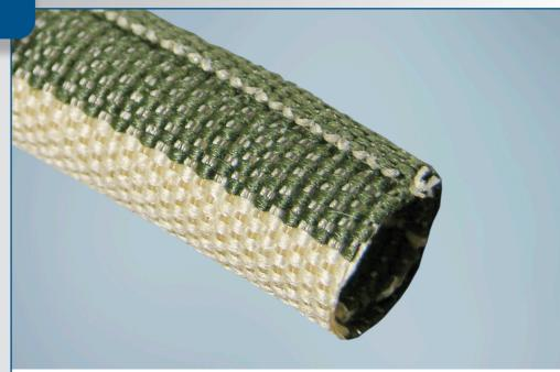
**ROUNDIT® 2000 NX HT** is a self-wrapping sleeve manufactured from PEEK monofilaments and Nomex® multifilaments. It includes a water repellent treatment in order to prevent the absorption of condensation build-up caused by the extreme changes aircraft are subjected to. Designed for mechanical protection and maintenance of wire and cable bundles, its 100% covering ratio provides excellent cut-through and abrasion resistance.
