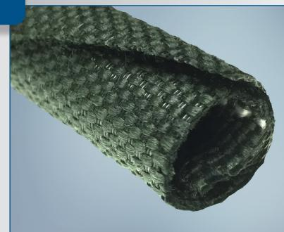
**ROUNDIT® 2000 NX** is a woven combination of Nomex® and PPS (polyphenylene sulfide). The Nomex®/PPS blend in a flat weave construction gives ROUNDIT 2000 NX a rugged yet smooth texture and appearance for high temperature bundling and abrasion resistance. This product is rated to +200°C (+392°F) and is non-halogenated.
