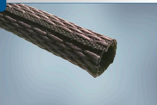
**ROUNDIT® 2000 FR GRIP** is a wrap-around sleeving manufactured from flame-retardant polyester monofilaments and multifilaments, designed for mechanical protection and maintenance of wire and cable bundles. Its construction with 100% covering ratio provides good abrasion resistance.
