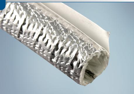
**ReflexWrap™ 1466** is a self-wrapping, reflective sleeve designed to provide thermal protection from both radiant and convective heat. Composed of a woven fiberglass base fabric and a lamination of aluminum foil, the product can withstand convective heat soaks and simultaneously protect critical components from radiant or reflected heat.
