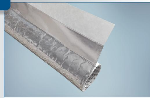
**ReflexWrap™ 1463 LF** is a self-wrapping, reflective sleeve designed to provide thermal protection for both radiant and convective heat applications. Composed of an aluminum foil laminated to a fiberglass woven fabric, the product protects critical components from radiant or reflected heat while withstanding convective heat soaks up to +200°C (+392°F).
