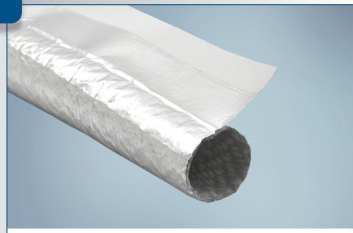
**ReflexWrap™ 1463** is a self-wrapping, reflective sleeve designed to provide thermal protection for both radiant and convective heat applications. Composed of a woven fiberglass base fabric and a lamination of aluminum foil, the product can withstand convective heat soaks up to +200°C (+392°F) and simultaneously protect critical components from radiant or reflected heat.
