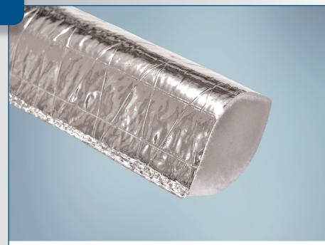
**ReflectSleeve® 1501** is reinforced, aluminized polyester sleeve designed to protect components in high temperature environments. The external surface is composed of a highly reflective aluminum foil, which provides radiant heat protection for internal components. The internal layer is composed of a polyester non-woven material, which provides added insulation efficiency. A layer of fiberglass scrim contributes to both product flexibility and durability.
