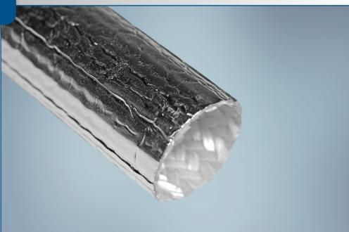
**ReflectSleeve® 1451** is a one-piece fiberglass sleeve that is laminated to an aluminum foil. A special manufacturing process permits the sleeve to boast a virtually seamless and non fraying construction. This feature makes ReflectSleeve 1451 a low profile solution easily applied to the application it protects. The outer aluminum finish is highly reflective while the inner layer of the fiberglass greatly increases insulating efficiency.
