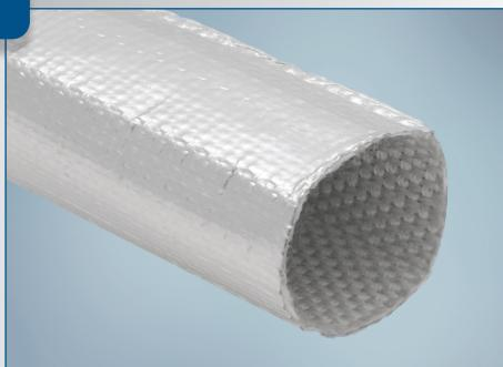
**ReflectSleeve® 1450E** is a woven, one-piece fiberglass sleeve that is bonded with an aluminized heat-seal film using a polymeric adhesive. A special manufacturing process permits the sleeve to boast a virtually seamless construction.
