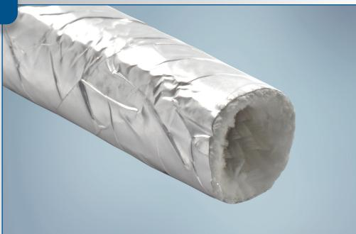
**ReflectSleeve® 1400** is a flexible, aluminized, high bulk, fiberglass sleeve used toprotect components in high temperature environments. ReflectSleeve 1400 features an outer layer of spiral wrapped aluminum foil that reflects radiant heat while providing a barrier against moisture and other damaging elements. The inner layer of high bulk fiberglass has natural air pockets which greatly increase insulating efficiency.
