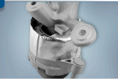
**ReflectShield® 1412** is a woven fiberglass fabric that has an aluminum foil laminated to its outer and inner surfaces. ReflectShield 1412 is designed to provide radiant heat protection for tubes, hoses, wire harnesses and other engine components.
