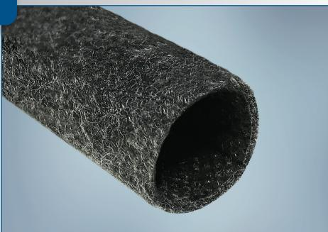
**QuietSleeve® 3008** is a tubular protective sleeve designed to provide excellent noise suppression and abrasion resistance. Composed of a non-woven polyester and polypropylene scrim, the product is lightweight and its thickness provides superior noise suppression performance for rattling/rubbing noise caused by vibrations.
