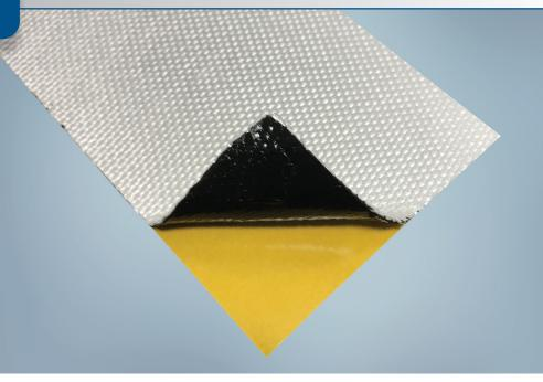
**Protexx-Shield® 7000 / 7005 / 7010** is a thin, flexible thermal and flame barrier specifically designed as anti-propagation protection within EV battery pack. Product is an engineered composite structure that provides functionality as a flame barrier and provides thermal insulation and electrical insulation. Protexx-Shield 7005 and 7010 is available with high temperature, pressure sensitive adhesive to allow for direct application onto a variety of surfaces.
