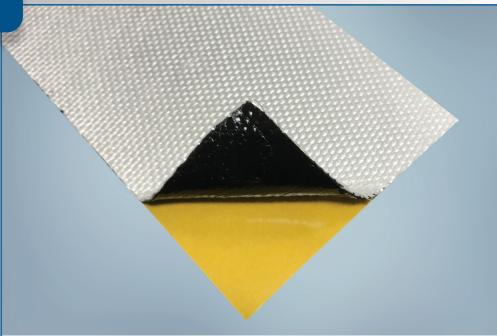
**Protexx-Shield® BP-B** is a thin, flexible thermal and flame barrier specifically designed as anti-propagation protection within EV battery pack. Product is an engineered composite structure that provides functionality as a flame barrier and provides thermal insulation and electrical insulation. Material is available with high temperature, pressure sensitive adhesive to allow for direct application onto a variety of surfaces.
