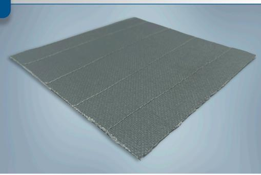
**Protexx-Shield® 7015** is a thin, flexible thermal and flame barrier specifically designed as anti-propagation protection within EV battery pack. Product is comprised of multiple layers of an engineered composite structure. Protexx-Shield 7015 acts as a flame barrier, low level blast barrier, medium level of thermal insulation and provides electrical insulation. Protexx-Shield 7015 is compatible with pressure sensitive adhesive to allow for direct application onto a variety of surfaces.
