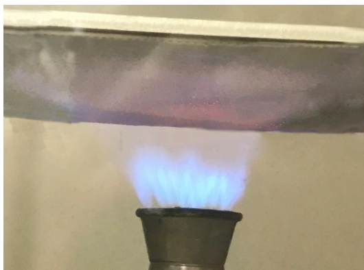
Flame test with Protexx-Shield® 3-Series
