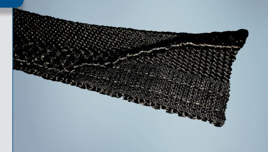
**ProGard® Wrap** is a durable, flame retardant, tightly woven nylon sleeving. Constructed from high denier nylon yarns, ProGard Wrap provides superior abrasion and cut-through protection for hoses, cables, wires, and other applications in a rugged environment. The hook and loop closure system allows for quick and easy installation.
