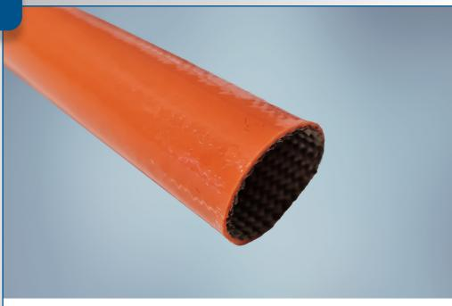
**HarnaSleeve® 1625** is a silicone coated fiberglass sleeve that electrically insulates wires to prevent arcing and short circuits. In addition, the sleeve's inherent thermal insulation and containment properties can be utilized depending on the application. The smooth, high gloss silicone creates a fluid tight barrier, provides additional protection, and is available in a variety of colors for identification purposes.
