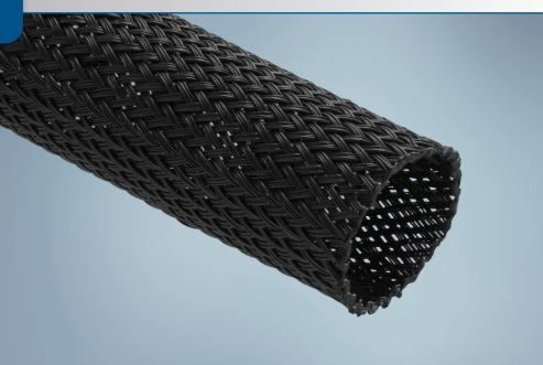
**FlexGuard® 2130** is a lightweight and flexible braided sleeve designed to provide mechanical protection for most common automotive applications. Constructed of PA (polyamide) monofilament guard strands and PET (polyethylene terephthalate) support strands, this dual-monofilament blend provides an excellent balance of abrasion protection, temperature resistance, and installability.
