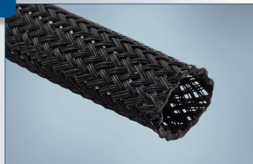
**FlexGuard® 2120** is a lightweight and flexible braided sleeve designed to provide mechanical protection for most common automotive applications. Constructed of PA (polyamide) monofilament guard strands and PET (polyethylene terephthalate) support strands, this dual-monofilament blend provides an excellent balance of abrasion protection, temperature resistance, and installability.
