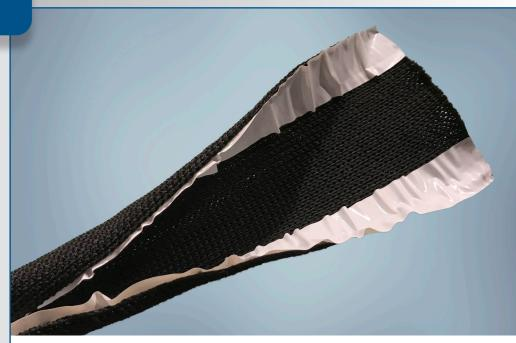
**FlexWrap® 3500** is a wrappable, damage-resistant sleeving designed to provide mechanical protection and acoustical noise suppression. Knit of monofilament and multifilament polyester yarns, the product offers a high level of component protection and is also very flexible.
