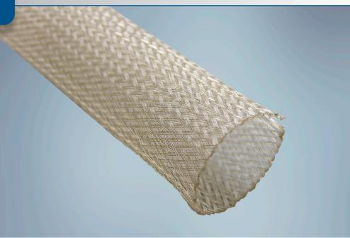
**Expando® 686DM** is an expandable oversleeve designed for mechanical protection in temperature extremes and hostile environmental conditions. Rated to +200°C (+392°F), Expando 686DM meets VW-1 and FAR Part 25 flammability requirements.
